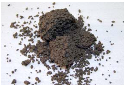
Decomposed "snow ball" due to too dry texture
