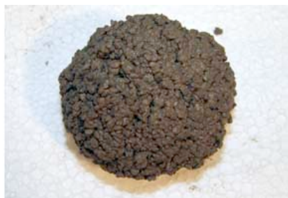
"Snow ball" at optimal earth-moist texture
