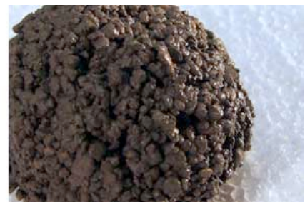
Binding-agent/water film on the surface of the "snow ball" at optimal texture.
