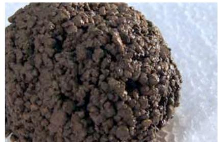
Binding-agent/water film on the surface of the "snow ball" at optimal texture.
